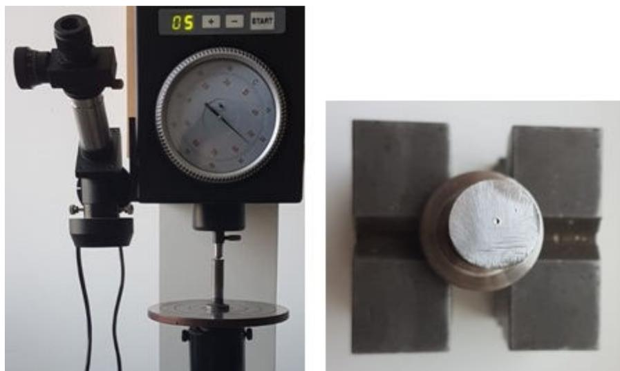
Figure 3. Hardness testing in the middle of tappet's rear (tail)
