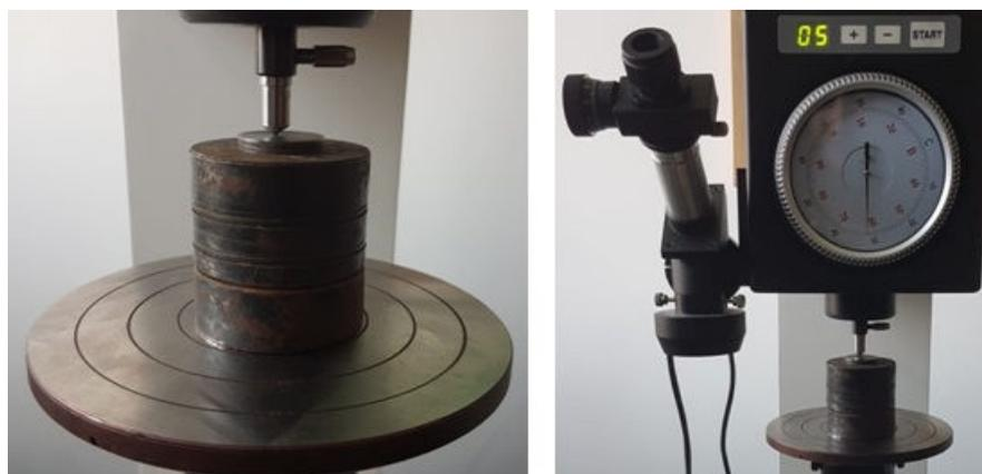
Figure 2. Hardness testing in the middle of tappet's plate
