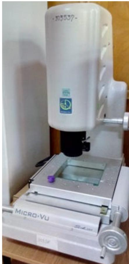
Figure 5. Coordinate measuring machine
