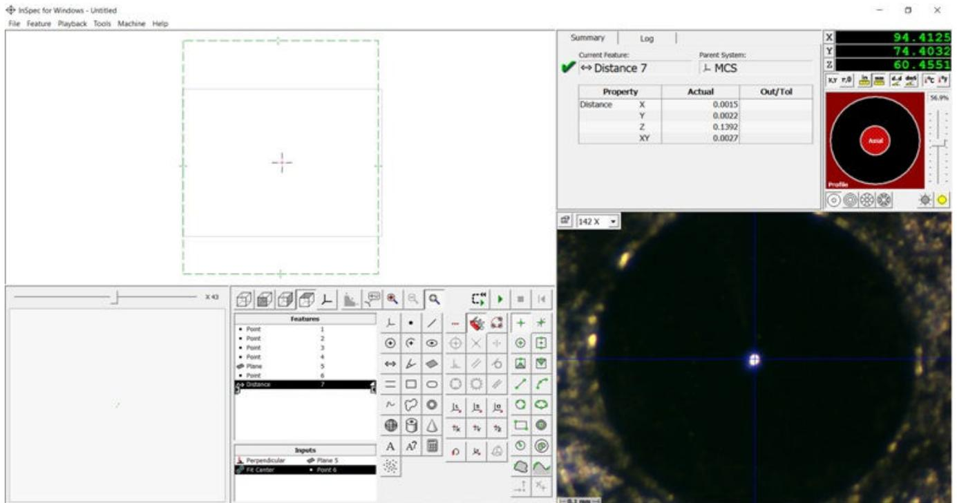
Figure 7. Indentation depth in one point on the exterior diameter of tappet's plate
