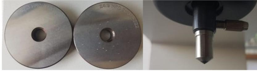
Figure 1.a) Reference sample HRC b) Conical diamond indenter
