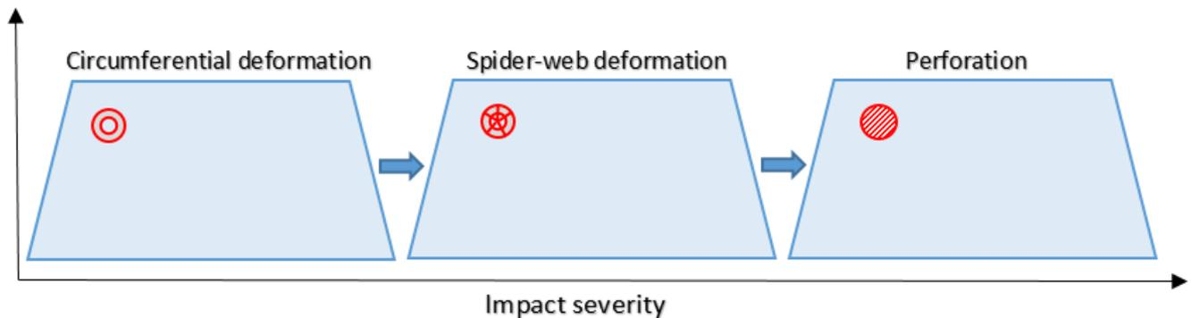
Figure 4. The stages of windscreen deformation [9]
