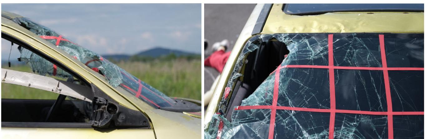
Figure 3. The windscreen perforation which resulted in the carried-out crash-test
