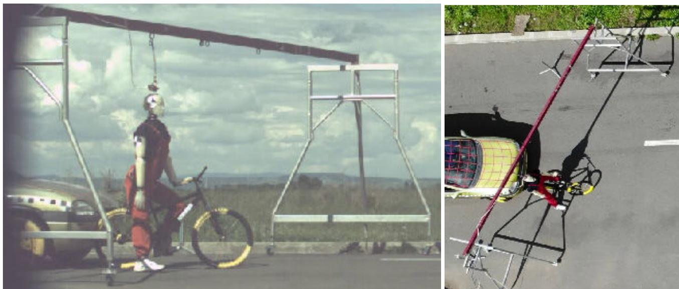
Figure 1. The crash-test scene and the gibbet support mechanism
